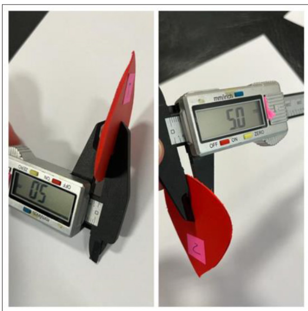
Figure 2: Central height of element 1 and 2 (Own source, 2022)
